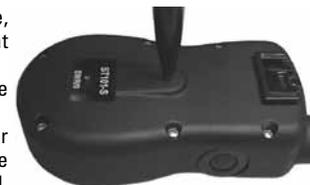
For example, if mode 5 is desired, adjust the Intensity Dial to Level 5. Once the mode button has been depressed, the Transmitter Indicator Light will be solid, and once the mode button is released, the Transmitter Indicator Light will flash 5 times. However, if you select mode 7 (ID Code), the light will remain solid in color once the mode button is released.
