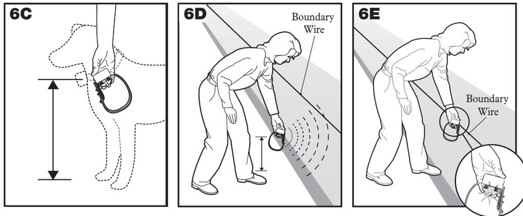
If the Collar Receiver does not beep at the desired range, adjust the Range Adjuster knob to the desired setting. Turning the Range Adjuster knob clockwise increases the Boundary Width while turning it counterclockwise decreases it. Repeat this activity as needed until the Collar Receiver beeps at the desired distance from the Boundary Wire.
