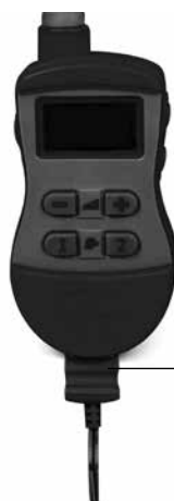
CHARGE CONNECTOR PLACED IN THE REMOTE TRANSMITTER CHARGING JACK
