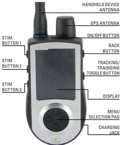
**HANDHELD DEVICE:** Receives and displays location updates from the GPS Collar. It is waterproof and can be submerged in water to a depth of 5 feet.
