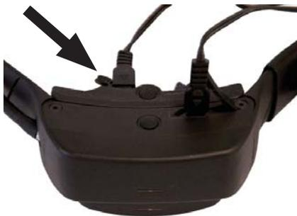
**Using Li-Ion technology, the E-Collar Module only requires a 2 hour charge. It is not harmful to let the unit charge more than 2 hours.**
